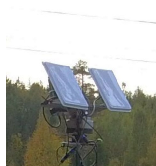
Automated directional UAV antennas
